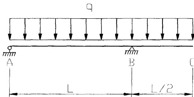
$$\begin{aligned}q &= 5 \text{ kN/m} \\l &= 8 \text{ m} \\A &= 20 \text{ cm}^2 \\I &= 2000 \text{ cm}^4 \\E &= 210\,000 \text{ MPa}\end{aligned}$$
