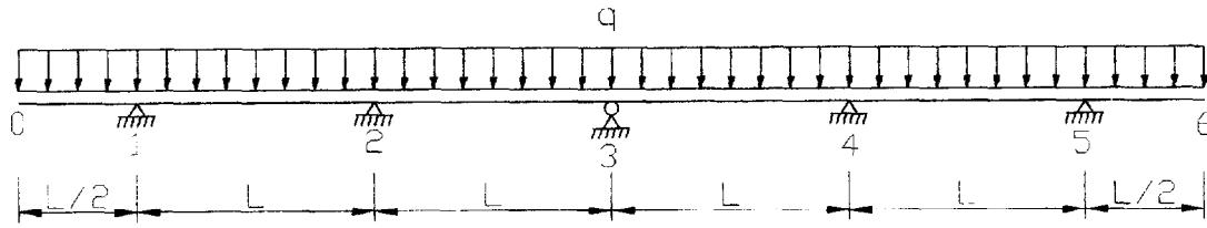
$$\begin{aligned}q &= 5 \text{ kN/m} \\I &= 8 \text{ m} \\A &= 20 \text{ cm}^2 \\I &= 2000 \text{ cm}^4 \\E &= 210\,000 \text{ MPa}\end{aligned}$$
